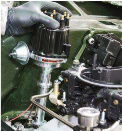
12 | Ignition comes from a fiercely reliable PerTronix billet street distributor with vacuum advance and the Ignitor III inside. The Ignitor III has all the advantages of the original Ignitor and Ignitor II, yet with a built-in rev-limiter.
