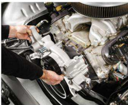
12 | The sophisticated water pump casting bolts to the block using OEM-style gaskets.
