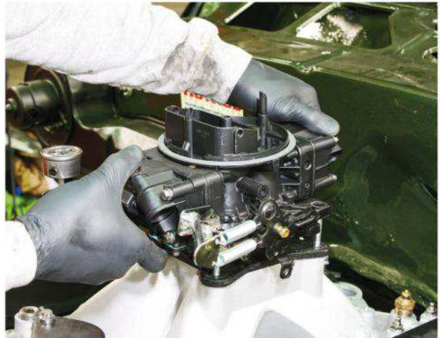
11 | Joel decided to take advantage of this engine bay update to also install an 800-cfm Holley carburetor and a tall, single-plane intake manifold.
