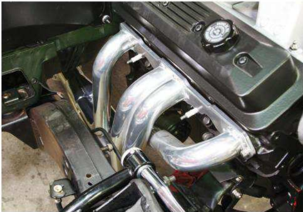
10 | The affordable Doug's long-tubes are a perfect fit, dropping cleanly inside the framerrails without interference issues. What's more, they do a nice job of exhaust scavenging, which nets more power. These tubes give Joel's Nova a nice throaty sound under acceleration.
