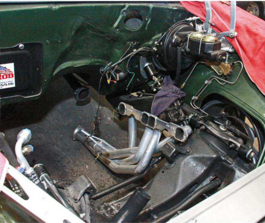
05 | Removing as many components as possible—especially the engine—makes it easier to do a professional job of detailing the engine bay. Joel took this thing down to the subframe and made everything like new again.
