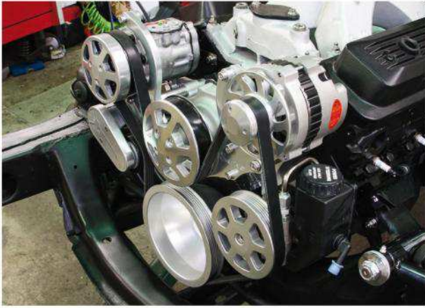
08 | Eddie Motorsports provided this complete serpentine drive system in billet aluminum. We like the compact nature of this system where nothing extends beyond the engine's perimeter.
