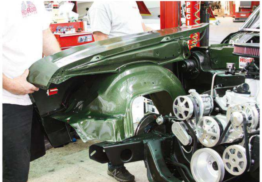
13 | The prepped and painted front fenders and wheelwells are carefully installed. It's a good idea to protect front end sheetmetal with blankets or towels. No matter how careful you are, there's always the risk of paint damage.
