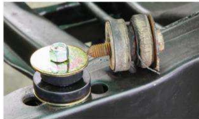
06 | Energy Suspension provided us with new polyurethane subframe mounts, which will isolate engine and driveline harmonics as well as road noise.
