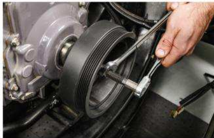
09 | We began the process by installing the Holley harmonic damper with a special tool we borrowed from our local auto parts store. (Don't try it without one or you could strip the threads inside your crankshaft.)
