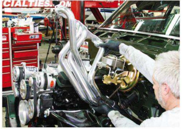
09 | The ceramic-coated, long-tube headers from Doug's Headers are a nice touch for this Nova's engine compartment. They're easy to install and the ceramic coating keeps destructive heat energy where it belongs.
