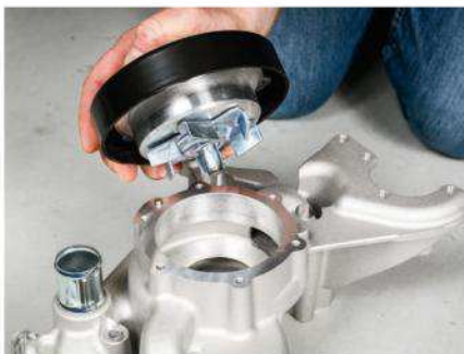
11 | The cartridge-style Holley water pump is a similar design to that used on the LT4 engine in the Corvette, though the two are not interchangeable. The internal ceramic seals are designed to survive sustained high-rpm operation.
