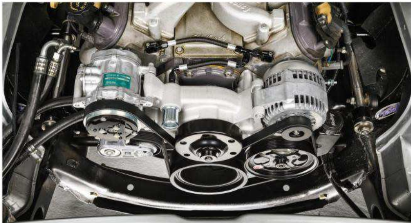
21 | The Holley Mid-Mount Complete Accessory System occupies virtually half the space used by the Corvette system.
