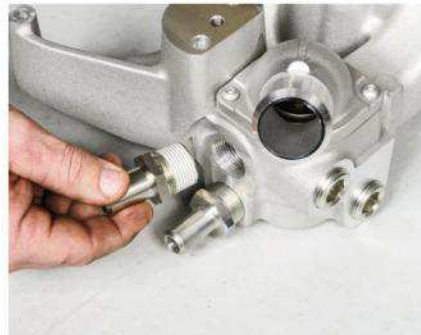
10 | The included thermostat housing and side heater hose ports worked best for the '69 Camaro.
