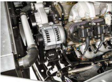
24 | There are now acres of space between the power steering pump and the upper control arm.
