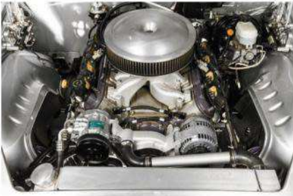
23 | With everything buttoned back up, the Holley Mid-Mount Complete Accessory System is right at home in the bay of this '69 Camaro.
